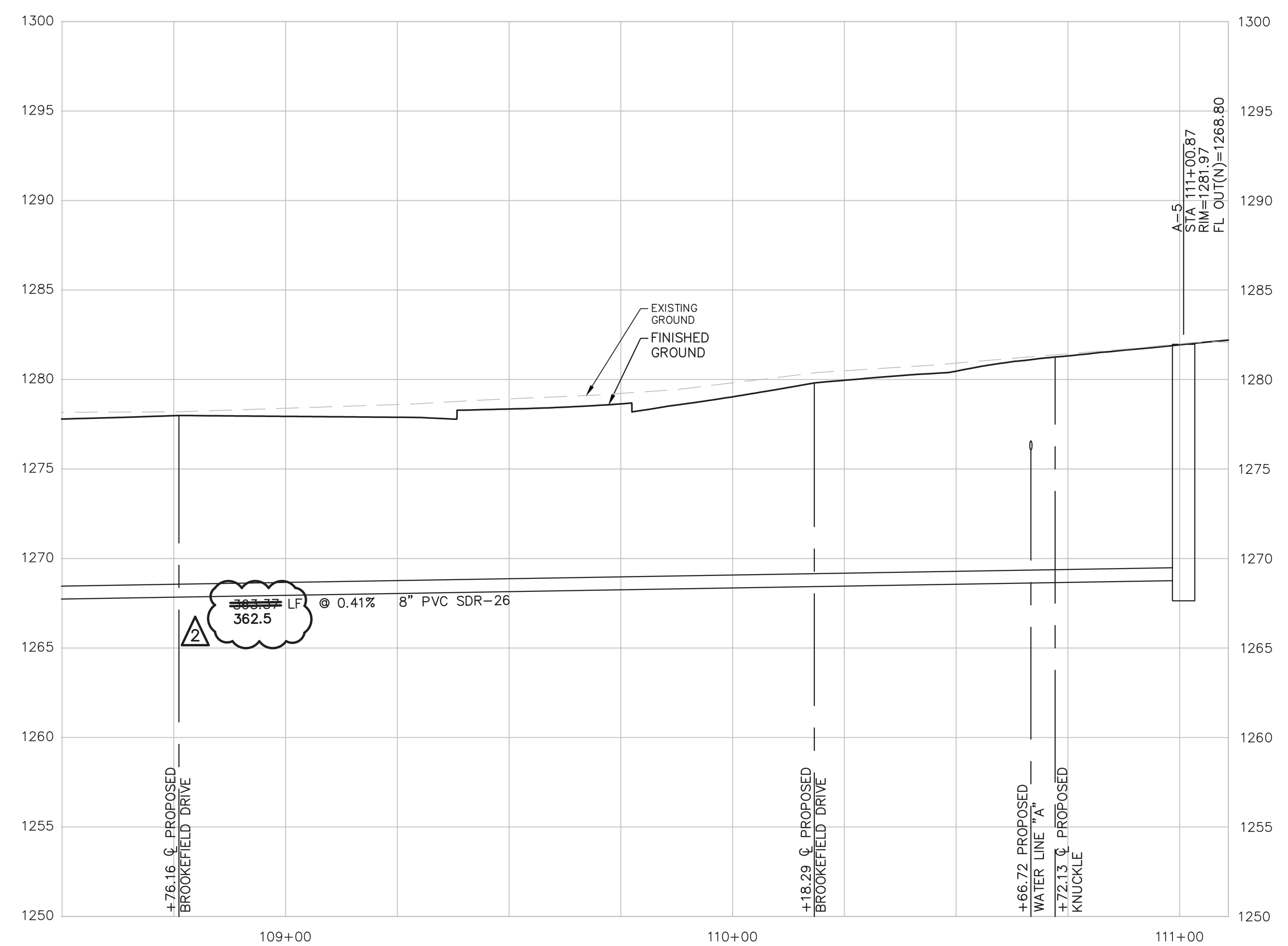
SANITARY SEWER LINE "A"
